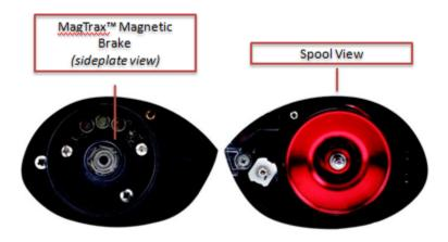
The *MagTrax*<sup>TM</sup> magnetic brake delivers consistent braking pressure throughout the entire cast resulting in smooth, controlled casts. A turn of the dial towards the "MAX" setting moves the magnetic braking system closer to the spool. As the magnets get closer to the spool, they apply more braking force and slow the rotation of the spool.
